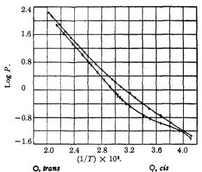
Graph showing variation of log of vapor pressure with reciprocal of temperature for isomers of decahydronaphthalene.
